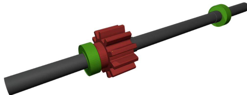
2x 3x6x2mm bearings and shaft has to fit tightly
