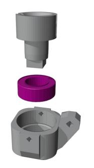
Bearings 5x8x3 has to fit very tight on axle. If axle is too big,
