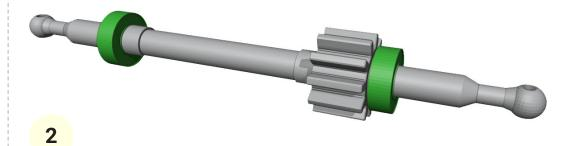
Bearings 3x6x2 has to fit tightly on axle.
