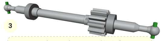
You need 2x 4mm long ~1.1mm thin wire (Best are paper clips.) and 3x 3x6x2.5mm bearings.
