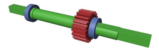
4x 7x11x3mm bearings has to fit tightly
