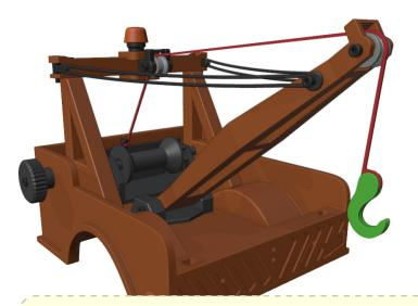
Tie the rope to screw and then screw it all the down. I recommend to use 1mm rope solft as possible.
